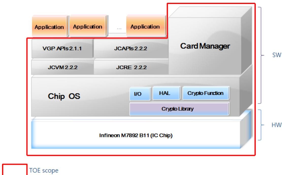
[Figure 2] Physical Scope of the TOE
